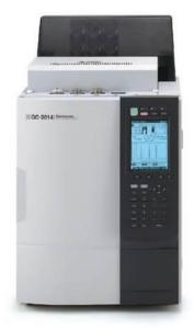
Gas Chromatography (GC) is a widely used analytical technique. It separates and analyzes volatile compounds in a mixture. The sample is vaporized and passed through a column, where different compounds interact with the stationary phase and elute at different times. The separated components are detected, quantified, and used for identification, making GC valuable in various industries such as environmental analysis, pharmaceuticals, and forensic science.
