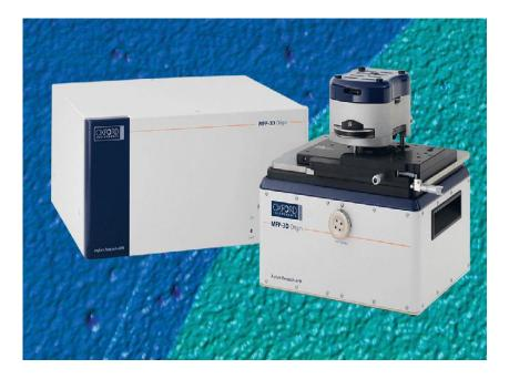
Atomic Force Microscopy (AFM) is a nanoscale imaging technique. It uses a sharp probe to scan the surface of a sample, measuring forces between the probe and the surface. AFM provides high-resolution topographic, mechanical, and electrical information about the sample
